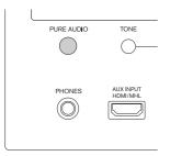
Selecting Pure Audio for listening mode turns off the display and analog video circuitry, but the video signals input through HDMI input are output from HDMI output.
